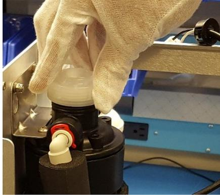
6. If a quartz tube is present, grasp the top of the tube and draw it out of the UV chamber by gently pulling upward. There are two O-rings which will likely come out with the tube. If the quartz tube is being installed for the first time, the two O-rings will be just below the white cap. Reach one finger into the chamber and lift out the two O-rings.
