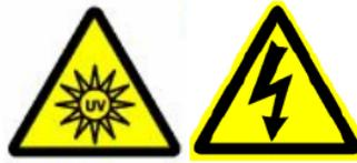
**WARNING:** Disconnect power to the WCS 2.0 before changing the UV lamp and follow the lamp replacement instructions. Exposure to UV light is hazardous to exposed skin and eyesight.
