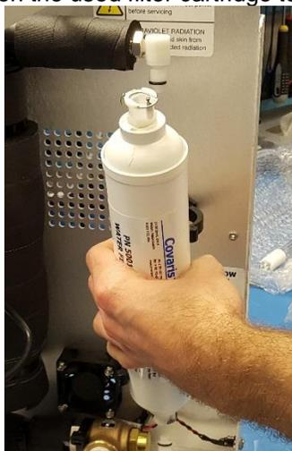
4. Install the replacement filter by pressing it down into the plastic grips, taking care that the flow arrows point towards the bottom of the WCS 2.0 cabinet. Reconnect the fittings as originally found by pressing them into each Quick Connect socket until they snap securely.
