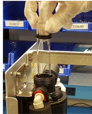
8. Thread the white cap onto the chamber by turning clockwise until snug. Hand tighten only.
