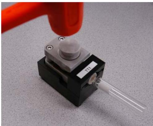
5. After impact, the pulverized sample can be transferred to the transfer tube. To do this, raise the cylinder with a gloved hand and remove the tissueTUBE.
