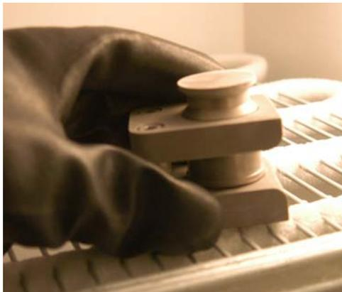
2. Place the pre-chilled portion of the CP01 cryoPREP Manual Dry Pulverizer into the holder (black piece) with the correct tissue tube adapter.
