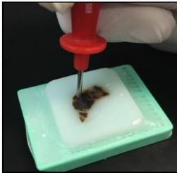
Loading Core Punch into microTUBE-500
