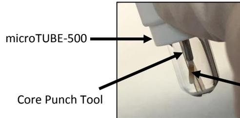
Core Punches Loaded into microTUBE-500
