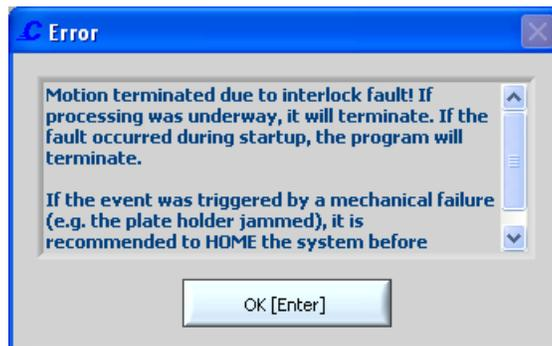
Figure 14 Interlock fault during method in progress
