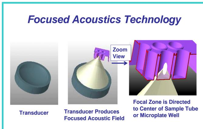
**Figure 3.** Diagrams showing "dish-shaped" Transducer producing Focused Acoustics Field creating a focal point at the top of acoustic field "cone" and directed inside Sample Tube or Microplate Well; this process produces energy for tissue homogenization
