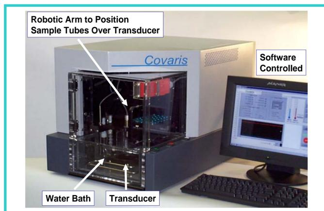
**Figure 1.** Picture of the Covaris E200 Focused Acoustics system. Sample tubes containing tissue sections in solution are positioned in water bath over Transducer one at a time for automated processing of up to 24 sample tubes in a single run
