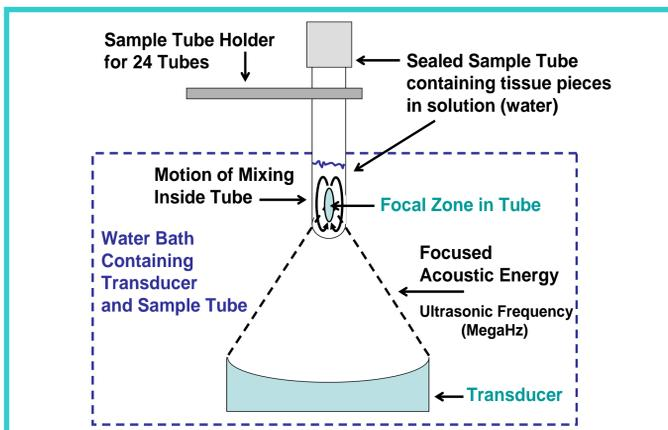
**Figure 4.** Diagram showing "cross section" of the Focused Acoustics tissue homogenization process; the Focal Zone located in the Sample Tube delivers the energy for tissue homogenization while simultaneously mixing the sample during the process
