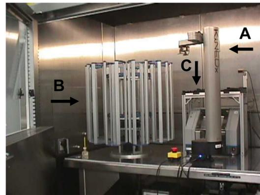
**Figure 2** System components include the Peak Robotics KiNEDx arm (A), a 10 position stacker carousel (B) and the delidding station (C).
