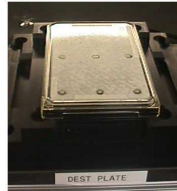
**Figure 3** Labcyte MicroClime lids prevent evaporation of DMSO from the destination plates and prevent hydration of the compound stock plates during extended automated runs.
