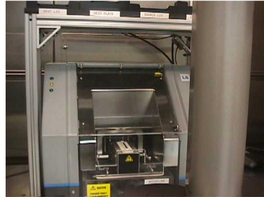
**Figure 1** Non-contact mixing is accomplished with the Covaris L8 Acoustic mixer. It can accommodate any microtiter plate as long as it is SBS standard footprint.
