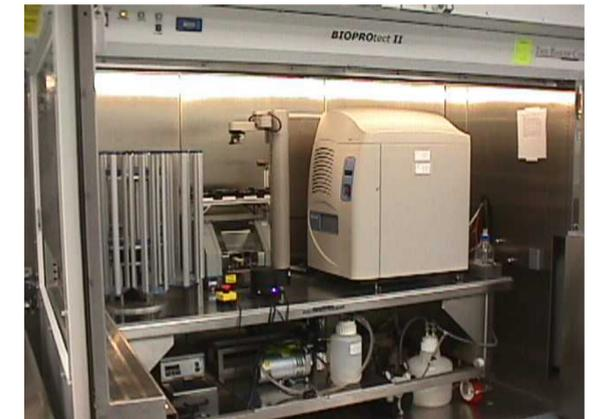
**Figure 5** The system as built and installed in the Southern Research Institute HTS Center. The system is housed in a Baker BioProtect II Biosafety Cabinet to maintain sterility or provide biological containment as required by the screen.
