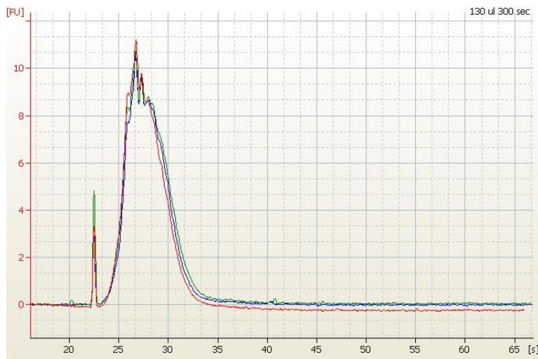
In three separate experiments 130  $\mu$ l RNA samples were sheared in a microTUBE AFA Fiber Snap-Cap using the following AFA conditions: DF 20%, PIP 50W, CpB 200 for 240 sec. Fragmented RNA was analyzed using Agilent Eukaryotic Total RNA Nano kit.
