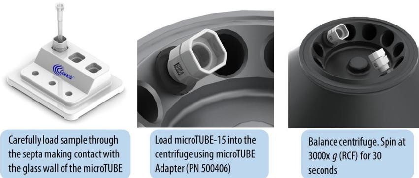
If some of the sample splashes onto the wall of the microTUBE while removing from centrifuge or placing into rack, repeat centrifuge step. All liquid should be at the bottom of the microTUBE-15 before starting the AFA treatment.
