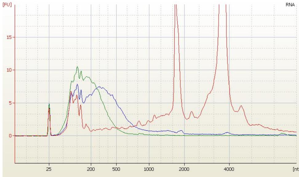
130  $\mu$ l samples of total RNA were treated in the microTUBE AFA Fiber Snap-Cap using the following conditions: DF 20%, PIP 50W, CpB 200 for, 0 sec (Red trace), 60 sec (Blue trace), and 240 sec (Green trace). RNA was analyzed using Agilent Eukaryotic Total RNA Nano kit.
