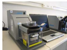
Figure 5. Covaris S-2 acoustic homogeniser with laptop control pc.
