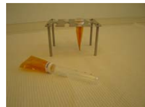
Figure 1. Covaris CryoPrep bag and a Cryobag sealed to a homogenisation tube.
