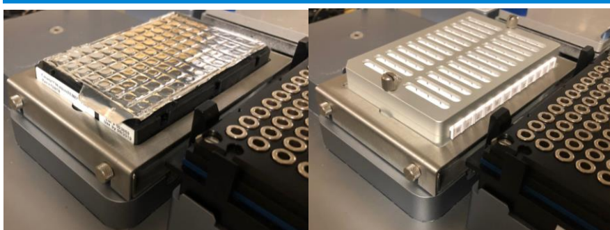
Figure 5 – Covaris Plate Adaptor with compatible consumables for the Agilent Bravo NGS and NGS Workstation. Plate adaptor assembly is comprised of three separate components: two base pieces secured by screws on CPAC base and one top piece that is height-adjustable and secured by four side screws. Adaptor is installed at Bravo Deck position 4. Configuration is adaptable for Covaris 96 microTUBE plates (A) and 8 microTUBE Strips (B).
