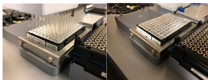
Figure 7 – Image of Covaris 96 microTUBE Plate being punctured by Agilent Bravo 96LT Pipette Head for sample transfer. A) Puncture of all 96 wells of a Covaris 96 microTUBE plate. B) Post-puncture view of a Covaris 96 microTUBE plate.
